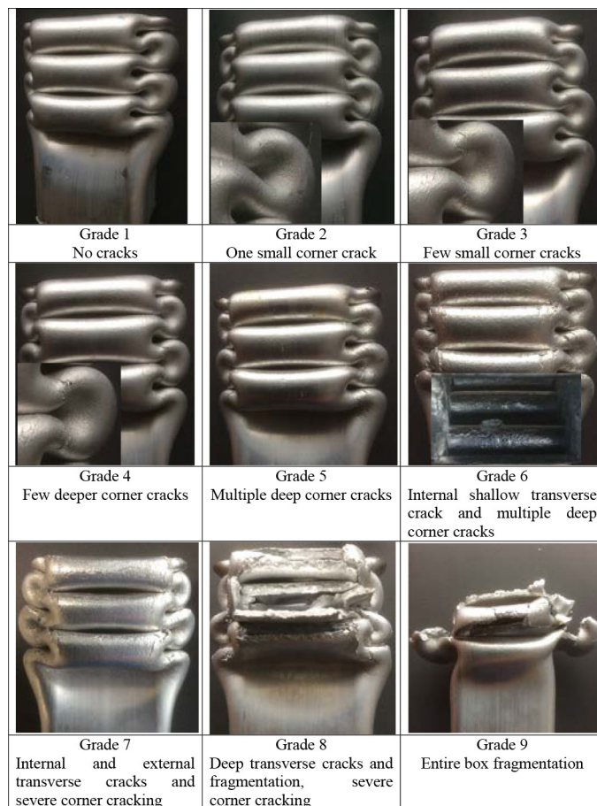
Figure 3. Crush grading system
